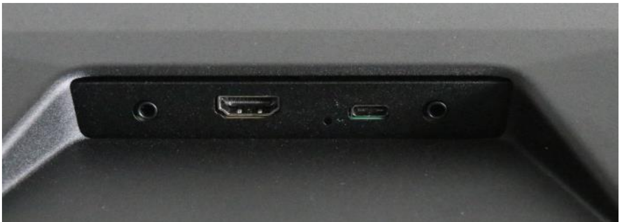
Input connectors customer: Headphone R - HDMI - USBC - Reset - Headphone L
