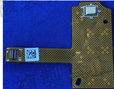
340-31974-000 ASSY, FPC, FRONT MIC AND MODE, CPPM1
