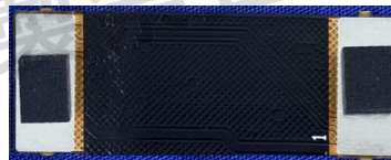
340-31973-000 ASSY, FPC, DISPLAY AND SHUTTER, CPPM1
