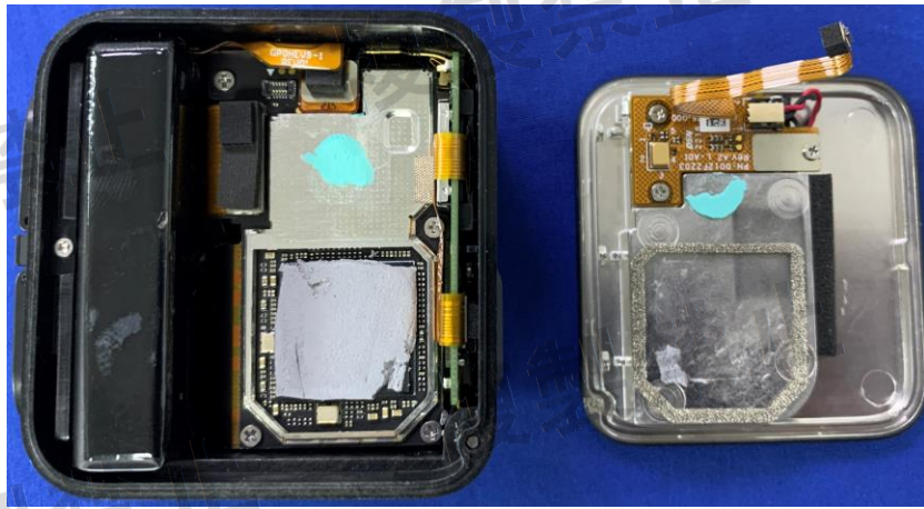
Rear cover, Mic, Speaker removed, CPPM1
