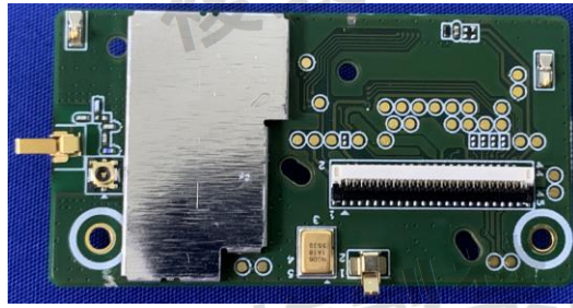
340-31977-000 PCBA, DISPLAY AND SHUTTER-Front with shield, CPPM1
