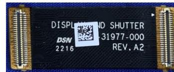
340-31973-000 ASSY, FPC, DISPLAY AND SHUTTER, CPPM1
