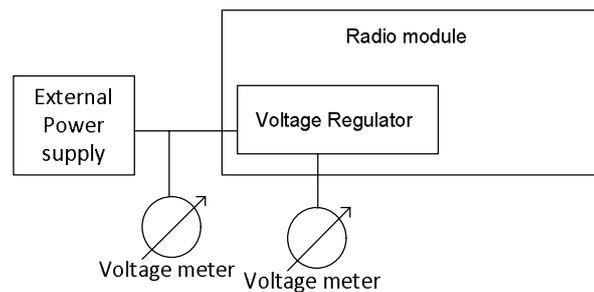
The extreme voltages were supplied by a laboratory power supply to the voltage supply pins of the module. The tests were carried out at a specially prepared EUT. At this EUT the power supply of the radio module and the output of the voltage regulator were connected by electric wires. While changing the voltage at the external power supply, the voltage variation at voltage regulator of the radio modules was measured.
