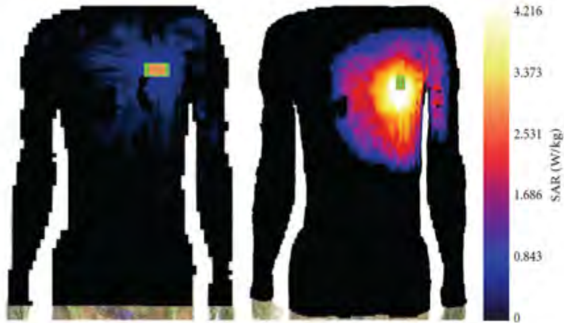
FIGURE 13: Simulated SAR values of two antennas on the body at 5.8 GHz: (a) reconfigurable beam-steering antenna, (b) loop antenna.
